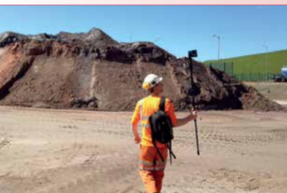
Fig. 5 - Stockpile scanning is made simple with the pole-mounted ZEB-REVO.
