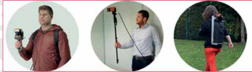
Fig. 1 - The ZEB-REVO in action – handheld, pole-mounted, backpack-mounted – a truly versatile tool.
