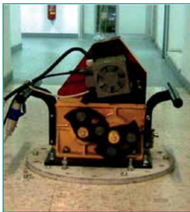
Fig. 11 – A vibrodyne used to apply an input to a building.
