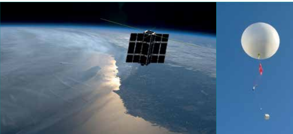
Fig. 5 - A radiosonde features a balloon and a payload capable of one vertical atmospheric profile/launch (right) and a LEMUR satellite (above) is capable of measuring 1000 atmospheric profiles/day.
