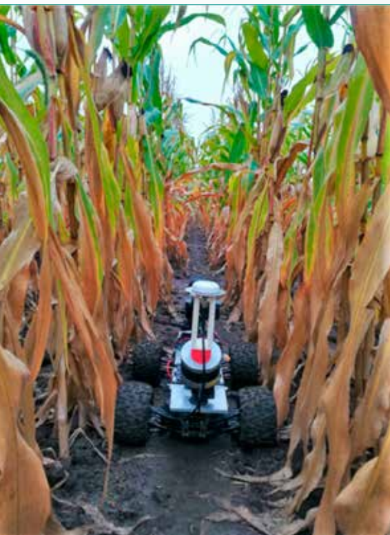
Fig. 1 - The mobile robot traversing under the canopy in a maize field (Manish et al., 2022).
