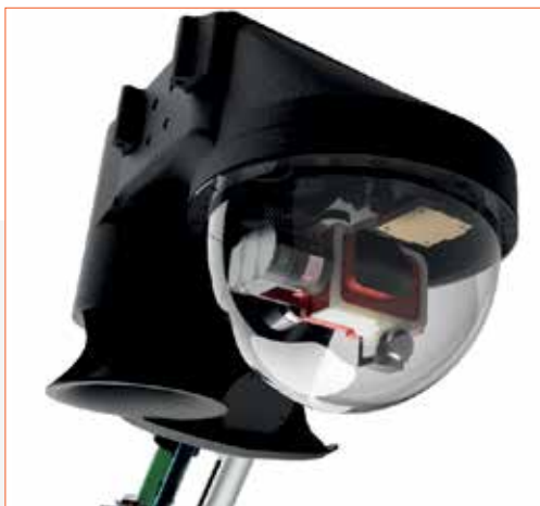
Fig. 7 - Multispectral camera and gimbal waterproof housing.
