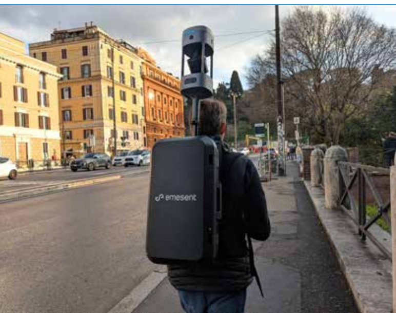
Fig. 3 - GX1 on backpack — surveyor in an outdoor AEC environment.
