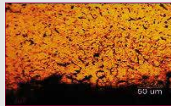
Fig. 3 - ME ex., for a sample from the spear a, shows crevice corrosion dispersed in the alloy.
