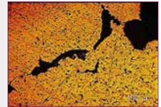
Fig. 4 - ME ex., for a sample from the spear b, shows the microcracks disturbing of the surface.
