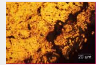
Fig.6 - ME ex., for a sample from the spear d, shows the crevice corrosion dispersed in the alloy.
