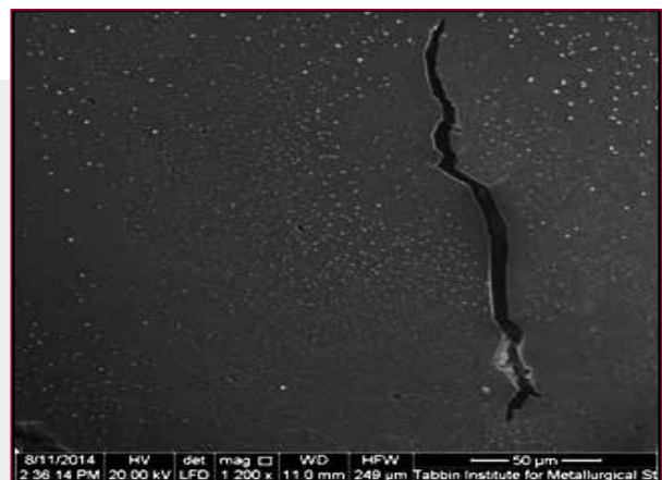
Fig. 5 (a, b) - SEM scan of the alloy shows the white block of zinc dispersed in the alloy and stress corrosion (a). A crossed section shows the stress corrosion caused micro cracks dispersed in the alloy (b).
